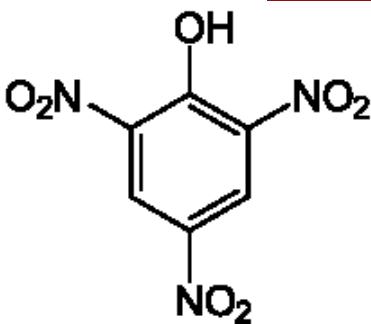
Fig. 1: Molecular structure of the picric Acid crystal
